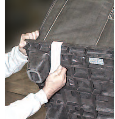
Pallet corner tie-down straps are used to secure the UniBin container to its pallet.
